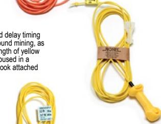
The NONEL EZ DRIFTER® system is used extensively in underground mining. EZ DRIFTER units consist of an out-of-hole detonator housed in a white plastic EZ Connector block on one end of a length of yellow shock tube with an in-hole detonator on the other end. Available in three standard delay combinations.
