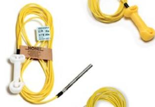
NONEL LP are in-hole detonators with a variety of precise long period delay timing and are extensively used in underground mining, tunneling, shaft sinking and special construction applications. These units consist of a long period delay detonator assembled to a length of sealed yellow shock tube with a blue plastic J-hook at the opposite end.
