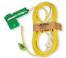
NONEL MS Connectors are used with detonating cord initiated blasts to provide millisecond delay timing between holes and rows. This bi-directional trunkline connector consists of an 18-inch (46 cm) length of shock tube with millisecond detonators of the same delay, inside color-coded connector blocks, on each end.
